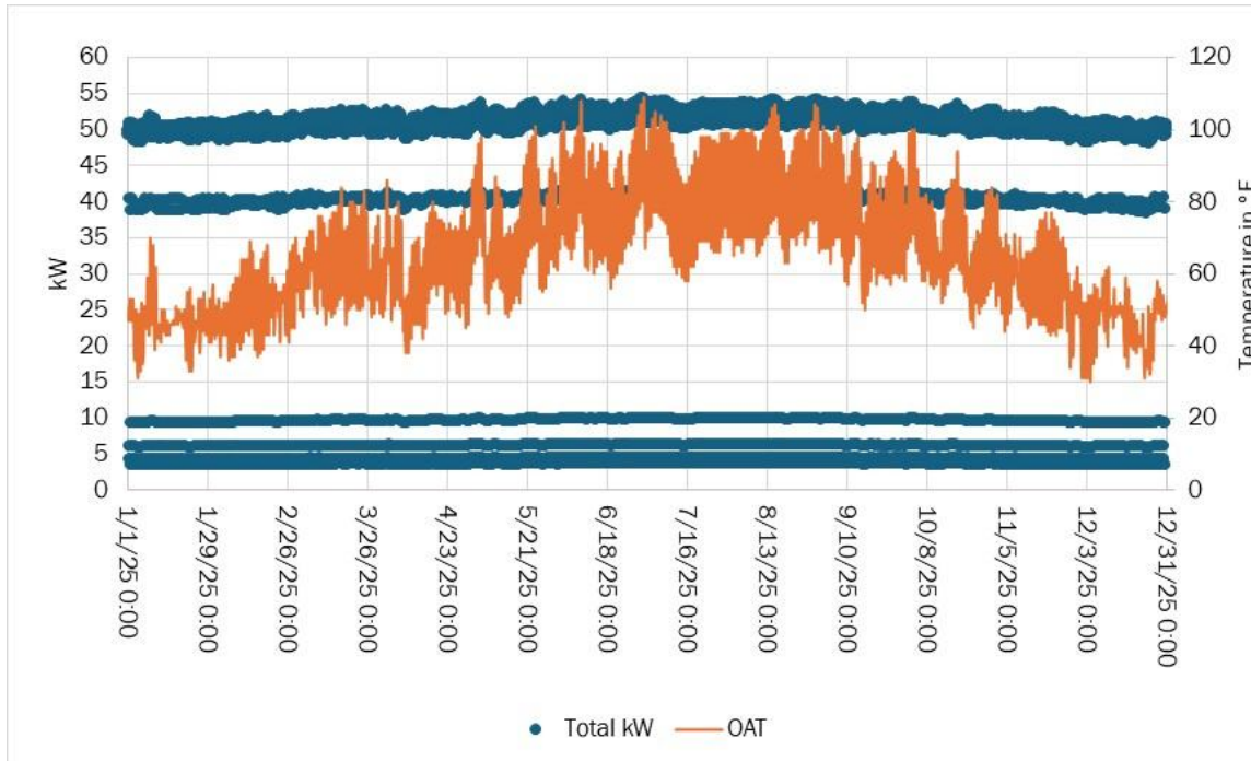
Figure 45: Normalized eastside chiller model using bin method.
